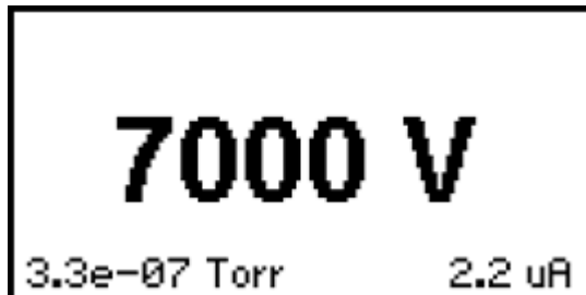
Figure 2. Display during ion pump operation
